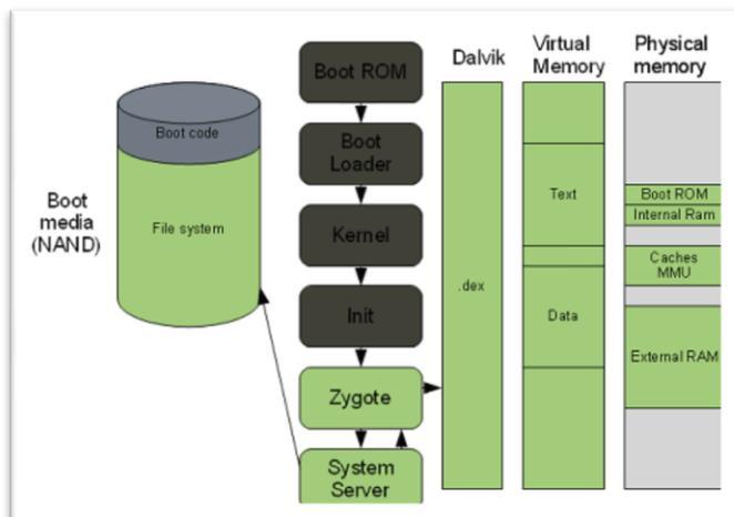
the Second Program Loader (SPL) to internal RAM and transfers execution to it. The SPL is in charge of loading the OS and other possible mode such as the Recovery partition or the Fastboot protocol. SPL copies the Linux kernel that is located on the boot media to RAM and then transfers execution to the kernel.
